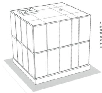
A 9,200 litre TIF tank shown mounted on a concrete slab base. This is one of the recommended methods of tank support structure suitable for TIF tanks.
